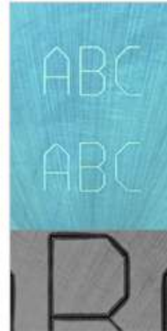
White marking (Evaporated by strong pulse)
